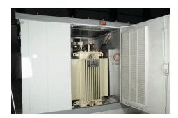
Designed in accordance with IEC 61330 standards, NIE's CSS is a prefabricated secondary substation with type-tested equipment and includes a distribution transformer, medium voltage switchgear, low-voltage switchboard, connections and associated equipment in a compact unit. Our CSS is designed keeping in mind high levels of personal safety and aesthetics as they are often located in high density, urban centres.
